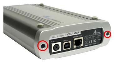
**Step 2** Pull out the front panel.
